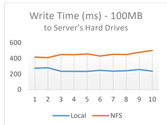
Fig 23. Write Time to Server's Hard Drive – 100MB data size
