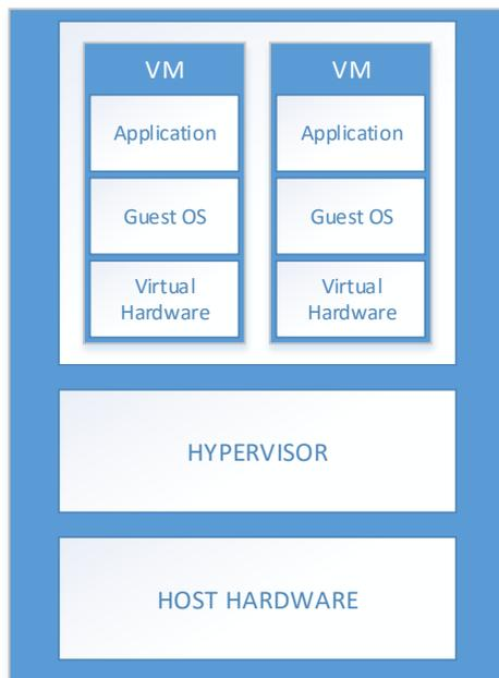
Fig 3. Architecture of bare metal hypervisor-based virtualization [1]
