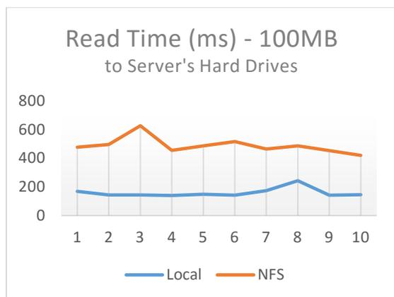
Fig 24. Read Time to Server's Hard Drive – 100MB data size
