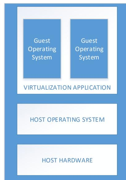
Fig 1. Architecture of operating system-based virtualization [1]
