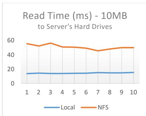
Fig 22. Read Time to Server's Hard Drive – 10MB data size
