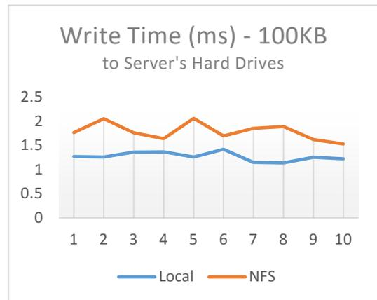
Fig 17. Write Time to Server's Hard Drive– 100KB data size
