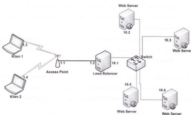
Gambar 10. Topologi Web server Load balance
