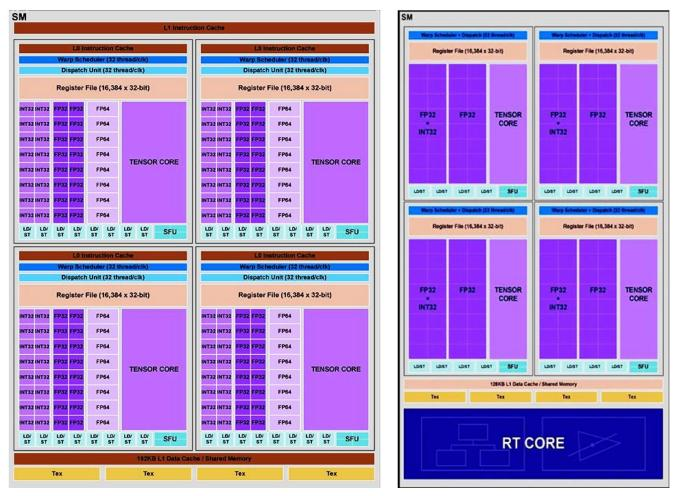
Figure 3. NVIDIA Ampere Streaming Multiprocessor Architecture [22]
