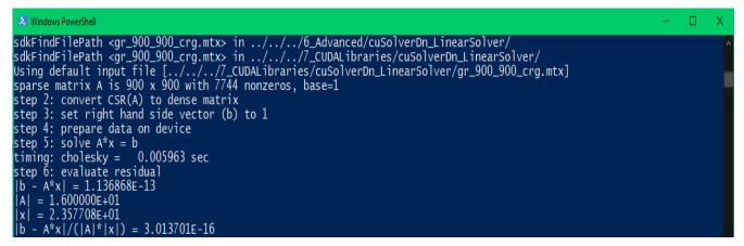
Figure 8. Solving a dense linear system using cuSolverDn
