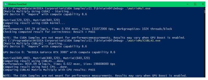
Figure 6. CUDA kernel and cuBLAS simple matrix multiplications
