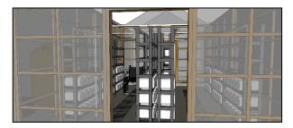
Fig. 4. The earliest structure proposal of the misting system for one level mushroom baglogs
