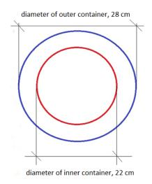
Fig. 5. Design of inner container diameter and outer container diameter
