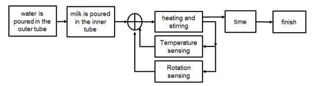
Fig. 4. Block diagram of milk pasteurization machine
