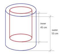
Fig. 6. Design of inner tube height and outer tube height
