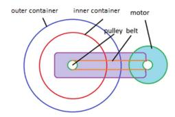
Fig. 7. The design of the stirrer motor position against the inner tube and outer tube
