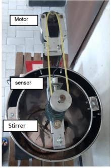
Fig. 8. Position of the stirrer motor to the inner tube and outer tube along with the rotation sensor
